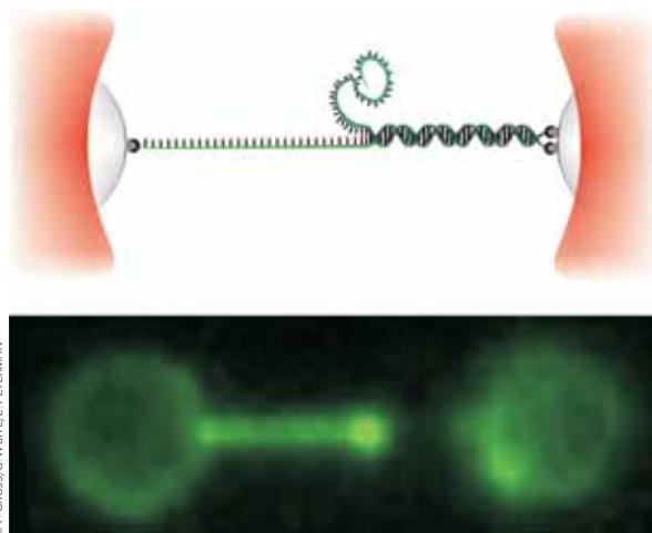
→ Top: Visual rendition of the experiment. The laser beams of the optical tweezers (red) hold the plastic beads to which a piece of DNA is attached and partially unzipped (left). Bottom: Fluorescent image of the process showing the two beads and the partially unzipped DNA (left).
